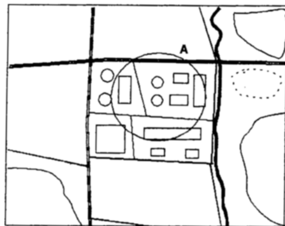
Fig. 9. Risk contours for scenario 6 indicating the impact area with 50 % probability of damage/lethality due to heat load (A).
