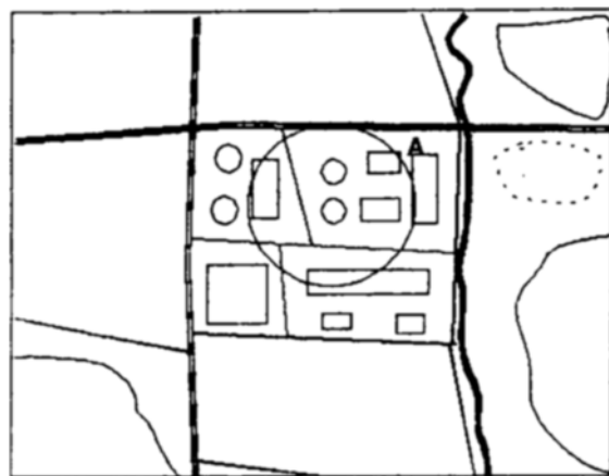
Fig. 10. Risk contours for scenario 7 indicating the impact area with 50 % probability of damage/lethality due to heat load (A).
